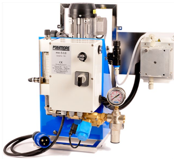
Figure 29. Flow-through polymer dosing unit 23
