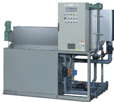
Figure 41. Compact installation of the disc press 28
