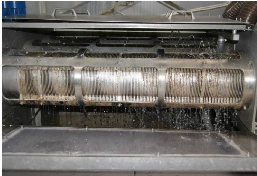
Figure 43. Disk press work area during dewatering process 30
